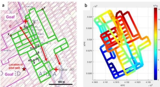
Figure 2a) Project example: Part of the mine plan under the Louisa Centre, Stanley, County Durham, UK. b) Modelling of the long-term mine water heating for this mine system through abstraction from the Hutton coal seam, and re-injection into a shallower seam.
