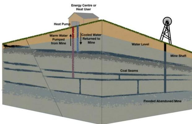
Figure 1) Schematic representation of a minewater heat pump system.
